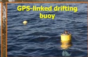
DMONs were deployed from GPS-linked drifting buoys. Two buoys with two DMONs each were deployed every day in the study area off El Hierro, Canary Islands.
